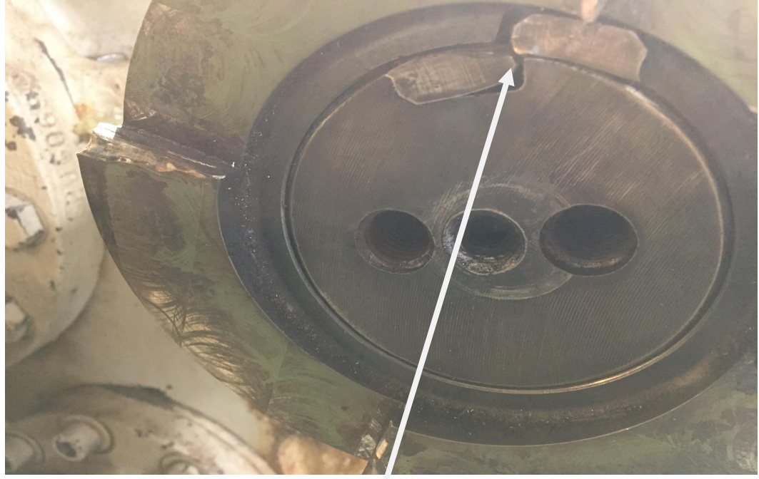
Jaw clutch hub on gear box side key sheared off & spun on shaft
