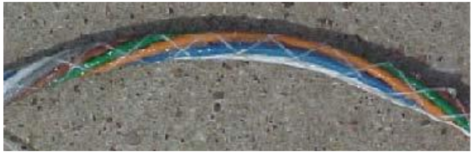
Figure 4: Reverse Spiral Wrap – Center of Exposed Buffer Tubes
